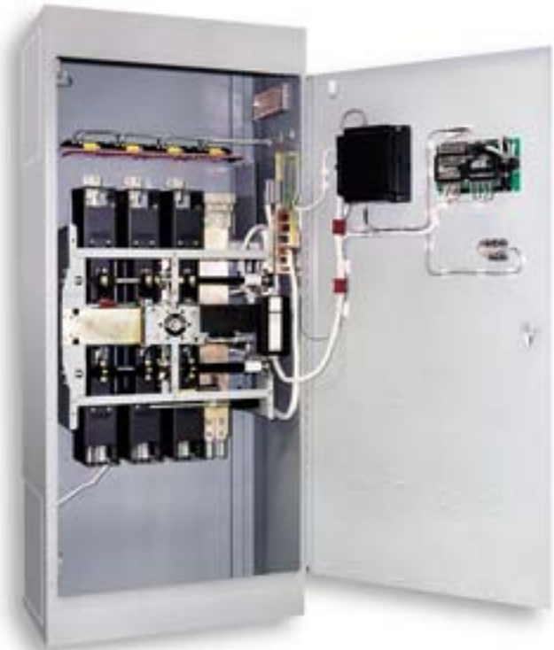
Fig. 1: Three Pole 7000 Series Automatic Transfer Switch rated 1600 amperes (shown with optional front connected terminals and Power Manager).
