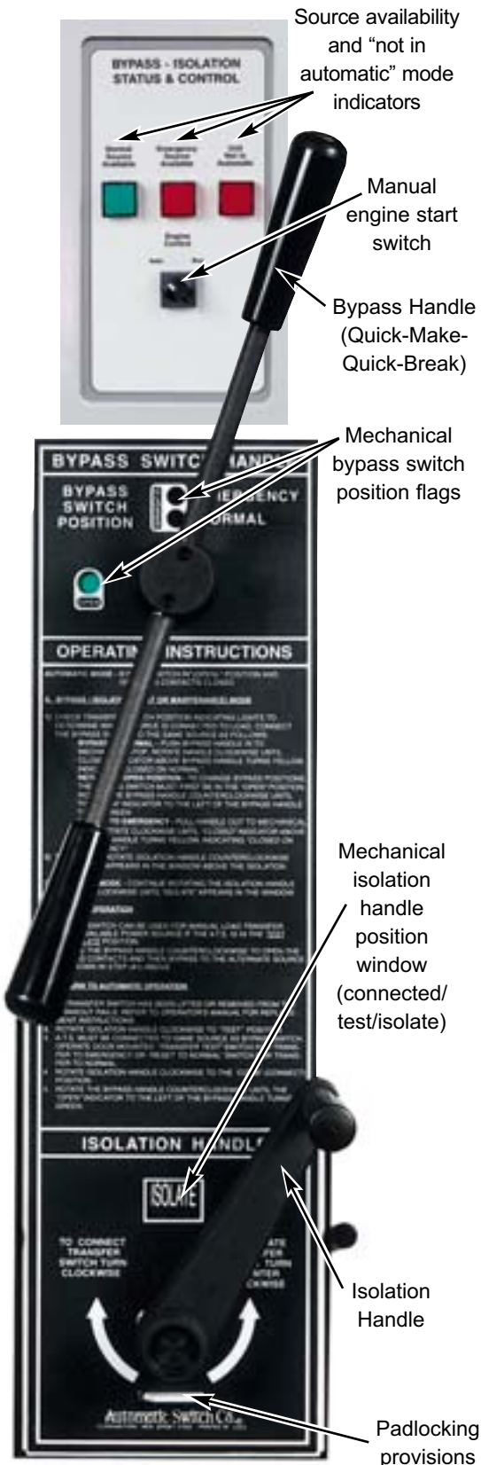
Fig. 8 Bypass-Isolation Switch user interface (1000-3000 amperes shown).
