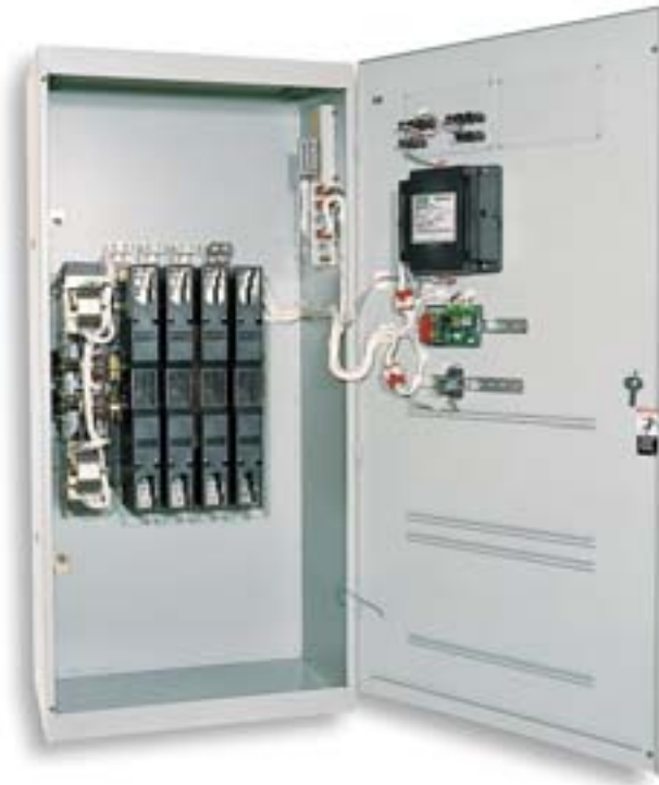
Fig. 2: Four pole, Closed-Transition Transfer Switch rated 1000 amperes in Type 1 enclosure.
